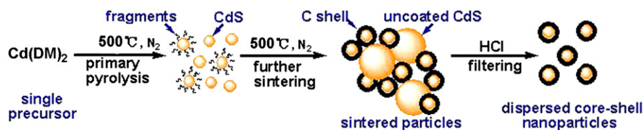
Fig. 6. Schematic illustration of the formation process of CdS@C QDs obtained from improved pyrolysis of Cd(DM) 2 .
